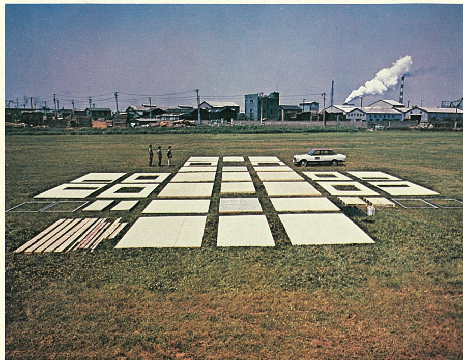
コアシステムの例(ホームコアの全部材) demonstrated panel inventory and finished materials for a unit of Misawa Homes' Core
