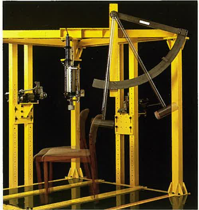
振り式衝撃試験 Impact Test by Hammer
